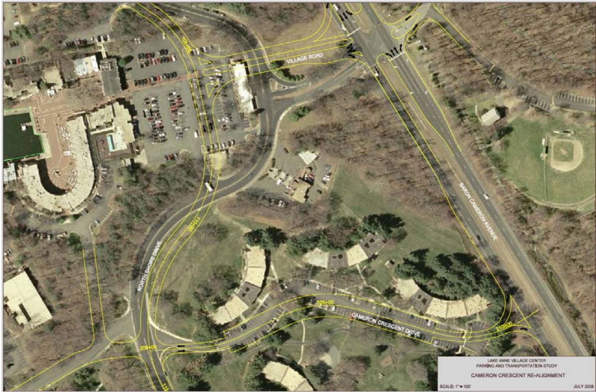
Figure 8 – Cameron Crescent Drive realignment and new intersection with Baron Cameron Avenue.
